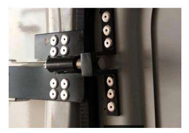
12/ If you have removed internal paneling to fit the Deadbolts you will need to cut out where the Deadbolts protrude through make sure there is room for the mechanism to operate.
